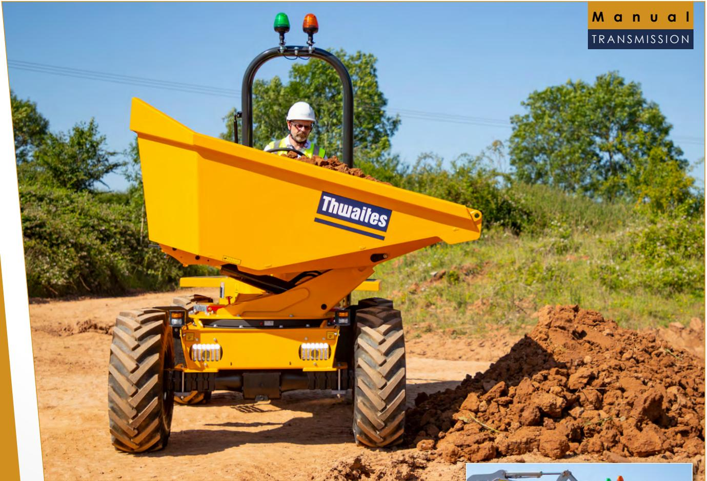
The Thwaites 3 Tonne Power Swivel, Stage V dumper is manufactured with contractors and hirers in mind – ensuring operator safety, reducing risk on site and improving performance. Powered by an 18.1 kW 3-cylinder Yanmar engine, delivering 107 Nm max torque for optimum traction and control. This machine is driven by a Manual transmission.
